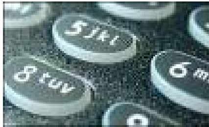
Figure 4. Mobile phone keypad on which alphabetic characters are added to each numeric key. Text entry is accomplished through repeated pressing of the numeric key. For example, entering the letter 'v' requires that the number '8' is hit three times.
