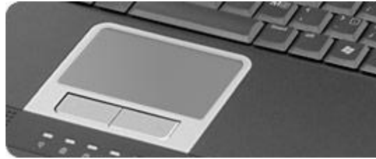
Figure 10. Synaptics touch pad. It senses a person's finger motion and translates the motion into a relative movement of an on-screen cursor .
