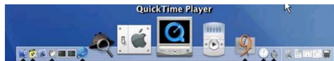
Figure 16. Tool dock in MacOS X. Commonly used tools are displayed with a larger icon to make selection time shorter. An additional configuration of the dock allows all icons to be the same size until the cursor passes over the dock. At that point, icons nearest the cursor are expanded.
