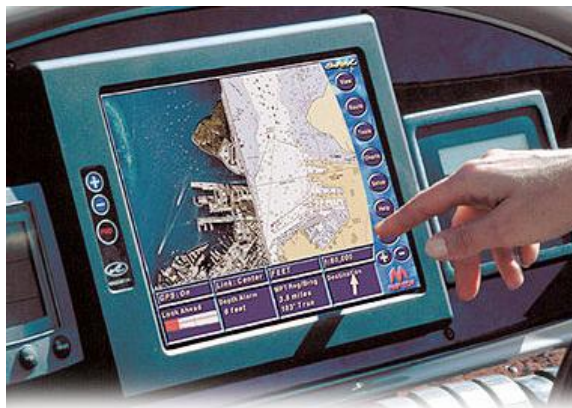
Figure 1. Maptech Sea Ray Navigator with 10" screen. The navigation menus are at the extreme right edge. The bottom of the display contains navigational data, including speed, current vessel position, and depth under keel.
