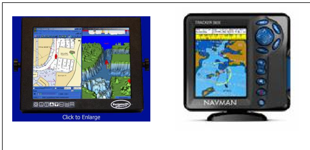
Figure 24. Examples of marine navigation systems. From left to right: Navigator Charting PC with Touch-Screen ECDIS, and Navman Tracker 5600 GPS and Chartplotter.
